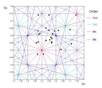
Figure 2: Working point diagram, showing cell tune flexibility for the TBA lattice, with emittance of 1.46 nm.
