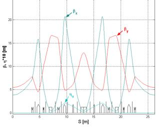
Figure 1: Lattice functions for 24 period lattice with  $\varepsilon_x = 1.46nm, (v_x, v_y) = (1.562, 0.560) / cell.$
