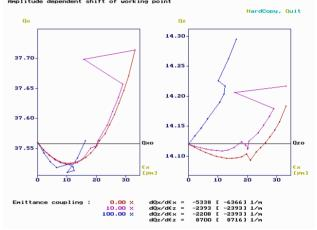
Figure 3: The betatron tunes Qx (left) and Qy (right) vs amplitude,  $\mathcal{E}_x = 2J$ , for 3 coupling ratios (0, 10, 100%) for the basic 24 period lattice with a 2<sup>nd</sup> order optimization using 7 sextupole families.
