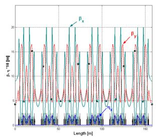
Figure 6: Lattice functions for a super period with 5 basic cells plus one high horizontal beta cell.
