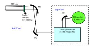
Figure 4: CSR power and spectrum measurement.
