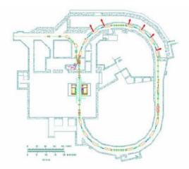
Figure 2: SHR ring plan view. Red arrows: IR beam line locations.
