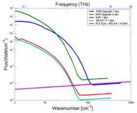
Figure 1: SHR CSR power spectrum horizontal acceptance/port: 300 mrad for upgrades, 60 mrad for all others.
