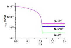
Figure 3: Time evolution of a normalized transverse emittance for different beam intensity.  $E_i = 400 \text{ MeV/u}$ .
