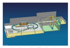
Figure 4: General layout of the CBS with rotating gantry.
