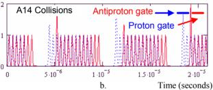
Figure 1. Proton (red solid) and antiproton (blue dashed) timing at A14 BPM for a.) acceleration and b.) collisions.
