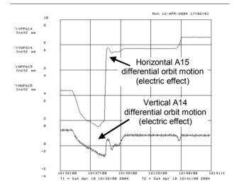
Figure 6. Horizontal and vertical differential orbit motion during low-beta squeeze. Vertical: 2 mm beam position per division. Horizontal: 60 seconds per division.
