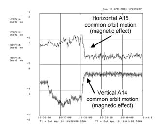
Figure 5. Horizontal and vertical central orbit motion during low-beta squeeze. Vertical: 1 mm beam position per division. Horizontal: 60 seconds per division.
