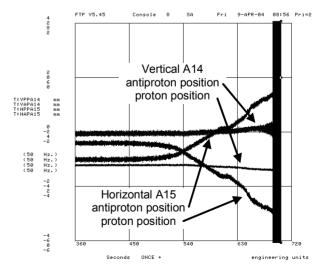
Figure 3. Horizontal and vertical proton and antiproton position measurements during separator scan. Vertical: 2 mm beam position per division all traces. Horizontal: 90 seconds per division.
