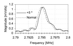
Figure 7: DSP based PSR frequency measurement for normal and +5 ° linac conditions.
