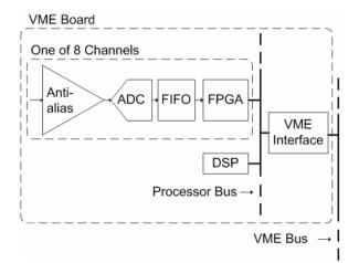
Figure 2: Board level architecture.
