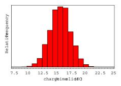
Figure 4: Noise distribution of the QIE front-end card (in calibration mode) with cable attached. The rms width of the histogram is 1.8 fC.
