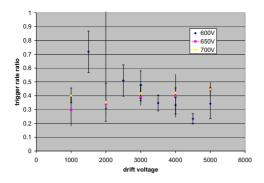
Figure 2: Electron detection rate with screening mesh divided by the rate without mesh, as a function of sweep voltage, for three different source settings (bias voltage on the Electron Generator Array).
