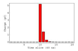
Figure 5: Test pulse injected into QIE front end card using laser-PMT charge injection system.
