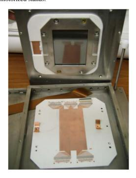
Figure 1: Partial assembly of detector, showing the anode board (bottom), MCP (top) and signal flex circuit (middle)
