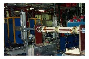
Figure 1: Modified air-core quadrupole on measurement stand in the Fermilab Magnet Test Facility.
