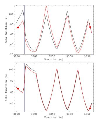
Figure 5: Fitted beta function in the e-sector. Top plot is horizontal, and bottom vertical plane. Red line is measured, black is design lattice. The dots are the data points, and the vertical lines indicate the location of the flying wires.
