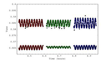
Figure 3: Measured tune variations on August 30, 2003. The E0 quadrupole was ramped 10 cycles first, then E17 and C0.
