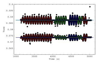
Figure 4: Measured tune variations on May 16, 2004. Red indicates E0 quadrupole ramping, green E17 and red C0.
