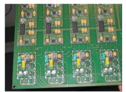
Figure 4: Picture of the four analog channels of the MPRX IV board. DC power supplies and the Bias voltage power supply are not shown.
