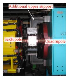
Figure 7: Additional upper support was fixed on a QM
