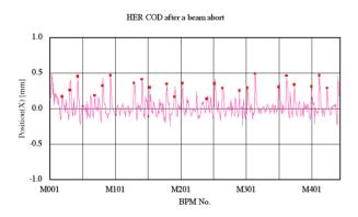
Figure 1: HER horizontal COD after beam abort. Red points are readings of BPMs located just down stream at the twin bending magnets.
