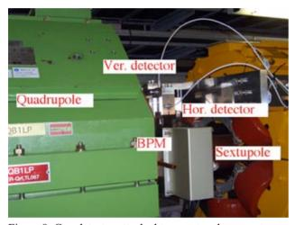
Figure 8: Gap detector attached to a sextupole magnet
