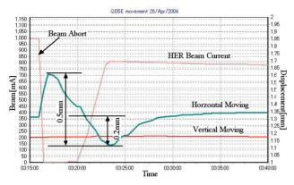
Figure 3: Readings of gap detectors after a beam abort.
