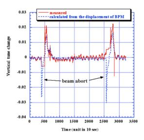
Figure 9: Vertical tune change calculated from the reading of the gap detectors and measured vertical tune change.
