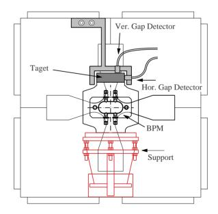
Figure 2: Gap detectors attached to QM
