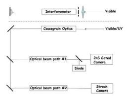
Figure 2: Single optical beam path for interferometer configuration (top) and dual optical beam path configuration (bottom). Reflective Cassegrain optics permits UV imaging on the CCD for improved resolution.
