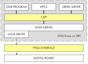
Figure 6: Software Architecture.
