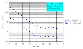
Figure 7: Resolution at two different bandwidths.
