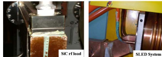
Figure 6: Water leaks at brazed joint (left: SiC rf load, right: SLED in linac).
