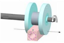
Figure 4: Two rotating aperture disks surrounding a crossflow tube that contains pressurized deuterium gas. The beam path is shown by the dashed arrow.
