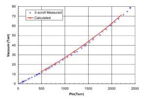
Figure 6: Plot showing the dynamic leakage of gas through the rotating aperture system compared to modeling (red line) Data is for helium gas and apertures set for a 2% duty factor beam.
