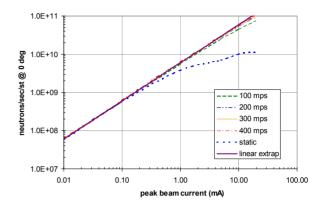
Figure 3: Predicted neutron intensity roll off as a function of peak beam current. Moving the gas from 100-400 m/sec in front of the beam decreases rarefaction.
