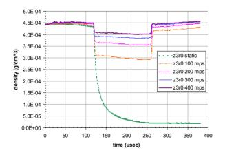
Figure 2: Density rarefaction due to beam heating in beam channel as predicted by hydrodynamic modeling. The step is the width of a macrobunch. The traces show the difference between static and moving gas.
