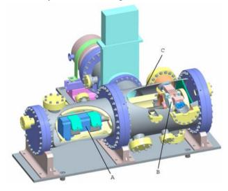
Figure 5: Details of the rotating aperture assembly including the motor (A), the cross flow tube and rotors (B), and the vacuum vessel (C). The overall length of the system shown is 1.2 m.
