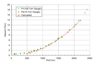
Figure 7: Static leakage results with the holes not aligned indicate the extent of leakage through the rotor-cross-flow gap compared to model (red line).
