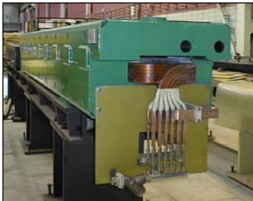
Figure 1: View of a 4 m long MSIB-module.
