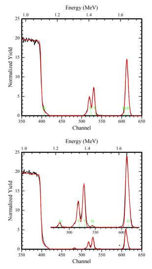
Figure 3: RBS spectra of Ti-Zr-V films using krypton (top) and argon (bottom) respectively as sputtering gas.
