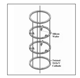
Figure 1: Silicon wafer sample holder for NEG film deposition. The assembly is mounted to the SST tube.
