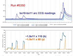
Fig. 3. Pressure rises (top) in the arc cold bore during 110-bunch proton (bottom) injections. The pressures were monitored with cold cathode gauges at room temperature connected to cold bore through a small conduit, resulted in readings a decade lower than the actual gas density in the cold bore.
