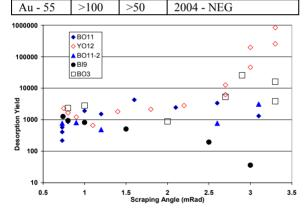
Figure 2. The Cu beam ion induced desorption yields from vacuum chamber wall vs. incident angles for stainless beam pipes (open markers) and NEG coated surface (filled markers) at single beam insertion regions. The effective desorption yields of NEG coated pipes are several times lower than the ones without coating.
