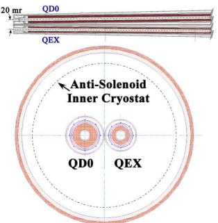
Figure 3: Side-By-Side QD0/QEX tapered cryostats, plan view (above) and section view in Anti-Solenoid (below).
