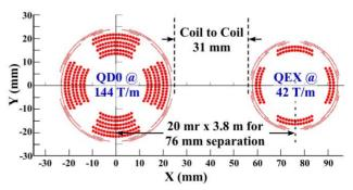
Figure 1: Cross section for side-by-side QD0 and QEX magnet coils at a distance of 3.8 m from the IP.
