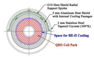
Figure 4:. QD0 Cryostat Detail at Support Location.
