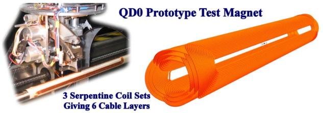
Figure 2: Start of winding for QD0 Prototype Test Magnet, QT, along with 3D view of the final coil configuration.
