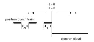
Figure 1: Schematic of the coordinate system for the positron bunch train and the electron cloud. The definition of the notations: s, z, l, and  $\Delta l$  are also shown.
