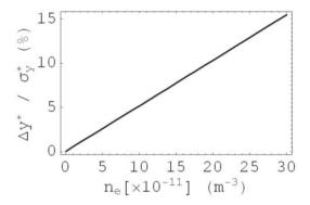
Figure 3: Effect of the beam-electron-cloud interaction for different electron-cloud equilibrium density  $n_e$  (m<sup>-3</sup>). The vertical axis is for  $\Delta y^*/\sigma_y^*$  at s=300 m, and the horizontal axis is the electron density.
