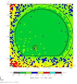
Figure 7: Muon flux isocontours on the detector.
