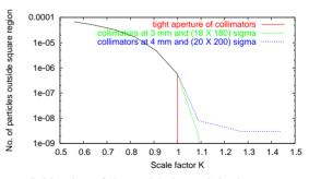
Figure 5: Number of charged-halo particles in a rectangular x-y window at the entrance to the final doublet.
