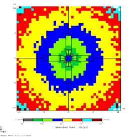
Figure 6: Absorbed dose isocontours in the quadrupole downstream of the mask PC1.
