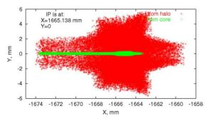
Figure 3: Transverse distribution of photons at IP from beam halo and core.
