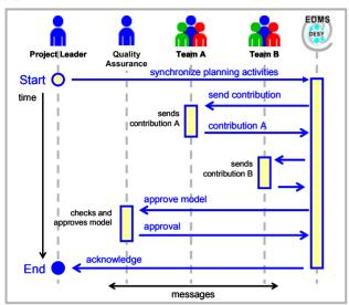
Figure 5: Process coordination using an Engineering Data Management System.
