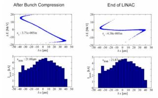
Figure 6: Longitudinal phase space and profile at exit of bunch compression system and end of linac from an 'elegant' calculation including all RF structure wake fields.
