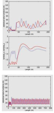
Figure 2: Space charge effects of 1 kA peak curent on optics downstream of compressor chicanes. Upper two pictures: optics and mismatch parameter downstream of  $1^{st}$  chicane (1 kA peak current, 500 MeV beam energy). Lower Picture: No effect downstream of  $2^{nd}$  chicane (5 kA peak current at 2.5 GeV). The red curves show parameters in the horizontal plane, the blue one in the vertical.
