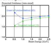
Figure 3: Projected emittance vs. beam energy (Strength of  $2^{nd}$  chicane bending magnets scales with energy).
