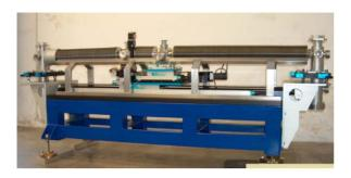
Figure 5: Emittance-meter device with long bellows.
