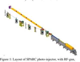
Figure 1: Layout of SPARC photo-injector, with RF-gun, 3 S-band accelerating sections and FEL undulator (6 modules). Beam line for undulator by-pass is also shown.
