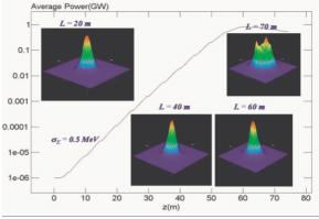
Figure 3: Power density profile along the undulator.
