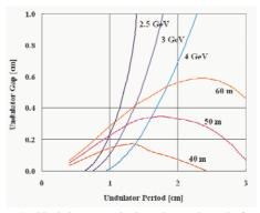
Figure 1: Undulator period and gap length for 0.3-nm SASE for saturation lengths (40, 50, 60 m) and beam energy (2.5, 3, 4 GeV).
