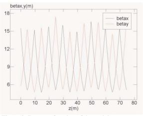
Figure 2: Betatron function of the undulator system.
