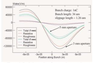
Figure 5: Resistive and surface roughness wakes.
