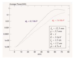
Figure 4: SASE performance vs. beam energy spread.
