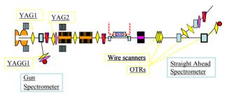
Figure 1: Layout of the diagnostics in the injector.
