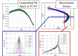
Figure 7: For nominal beam conditions in the transverse plane but with the uncorrelated energy spread increases from 0 to 50 keV - (a) Longitudinal Phase Space at the transverse cavity location –(b) XY image at spectrometer screen- (c) Evolution of vertical slice –(d) Evolution of horizontal slice.
