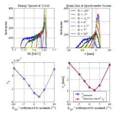
Figure 4: 1<sup>st</sup> column Projection of energy spread at YAG1 – 2<sup>nd</sup> column Horizontal profile at spectrometer screen.
