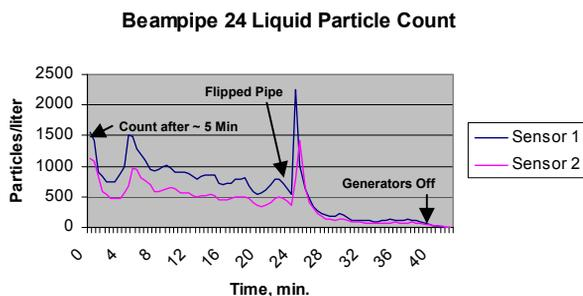
Figure 6: Liquid particle sampling of warm section ultrasonic cleaning.
