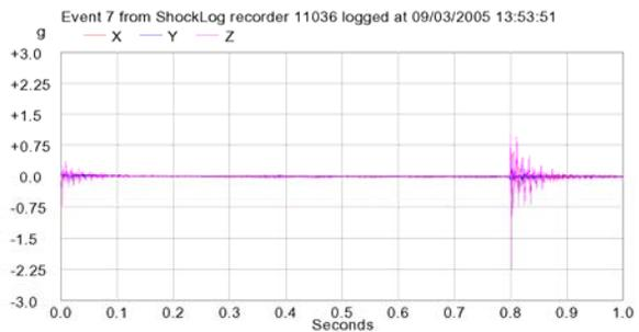
Figure 2: Most severe transportation shock – experienced during cryomodule offloading.
