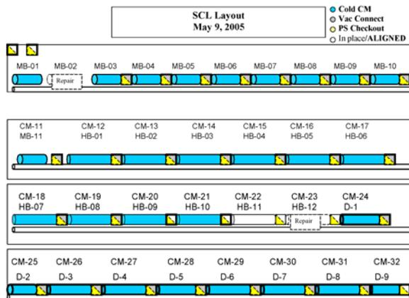
Figure 8: Installation Progress Chart.
