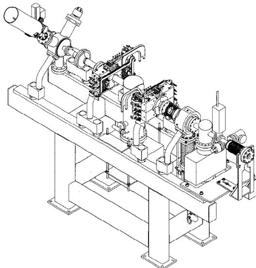
Figure 7: Low Energy Differential Pumping Station.
