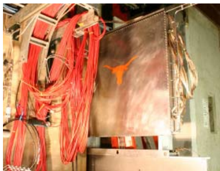
Figure 3: The hadron monitor during installation into the beam absorber. The monitor is installed on rails through a 2m(H)×15cm(W) slot in the concrete shielding.
