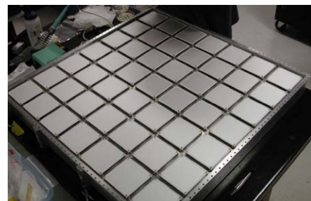
Figure 2: The hadron monitor during assembly showing the 7 \times 7 array of ceramic ion chambers.
