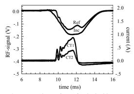
Figure 3: Measured waveforms for the incident RF-power (Inc) and the reflected RF-power (Ref) at the RF-gun, the current monitor after the gun exit (CT1), and after  $\alpha$ -magnet (CT2).
