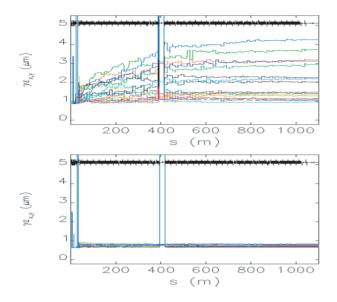
Figure 4: Normalized emittance along linac with a 1-nC (top) and 0.2-nC (bottom). The linac quadrupoles, BPMs, and RF structures are all misaligned by 250  $\mu$ m rms and the trajectory is corrected for 10 different seeds.
