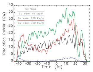
Figure 6: *Ginger* FEL calculations of the 0.2-nC case, including resistive wakefield losses along the undulator and various magnetic field tapers to optimize the power.
