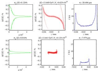
Figure 3: Longitudinal phase space in FEL at 13.6 GeV with 1-nC (top) and 0.2-nC (bottom). Plots show the energy profile (left), phase space (center), and longitudinal distribution (right). Bunch head at z < 0.
