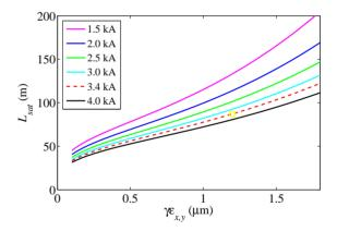
Figure 1: SASE saturation length [3] at 1.5 Å as a function of transverse emittance for several values of peak current.
