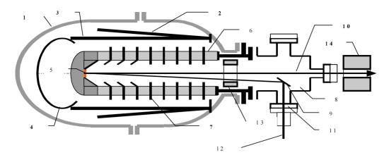
Figure 1: Schematic shape of the accelerator of electron bunchs with photocathode. 1 - tank for gas, 2 - primary winding of the pulse transformer, 3 - secondary winding of the pulse transformer, 4 - high-voltage electrode, 5 - photocathode, 6 - isolation rings of accelerating tube, 7 - electrodes of accelerating tube, 8 - vacuum chamber, 9 - mirror, 10 - electron beam, 11 - vacuum tube, 12- laser beam. 13- magnetic focusing lens, 14 - electromagnetic focusing lens.
