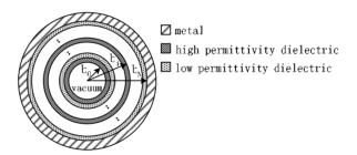
Figure 1: Cross-section of the general multilayered DLA structure.
