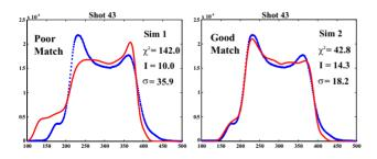
Figure 2: Example of a poor and a good fit. The only difference in the simulations is that overall rf phase changed by 0.5 degrees. Our method is sensitive to small changes.
