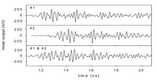
Figure 4. Experimental results using the new AWA gun and linac to excite a wakefield using a two bunch train. Each bunch has an intensity of 15 nC. #1 is the wakefields of beam 1 alone, #2 of the beam 2 alone, #3 wakefields of the two bunches simultaneously.
