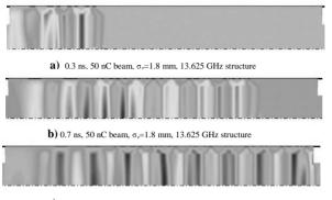
c) 0.9 ns, 50 nC beam,  $\sigma_z$ =1.8 mm, 13.625 GHz structure
