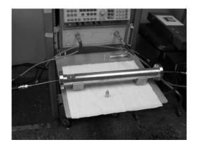
Figure 1. Bench test of the 13.625 GHz dielectric based accelerating structure at Argonne Wakefield Accelerator, Argonne National Laboratory.
