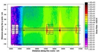
Figure 1: Remanent dose rate distribution after 180 days of continuous operation and one day of cooling period shown for a horizontal cut through the geometry at the height of the beam axes.
