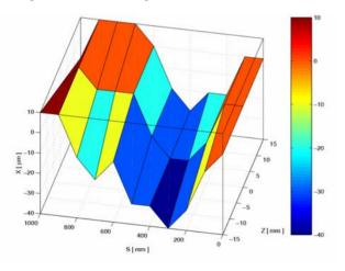
Figure 3: Flatness of the fully assembled CC jaw over its 1m long (S) flat top and for three positions along its width (Z). This was measured after bake-out at 250 °C.
