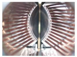
Figure 2: View along the free beam path of the CC collimator with a small collimation gap (~2 mm). The RF contacts guide the beam image currents.
