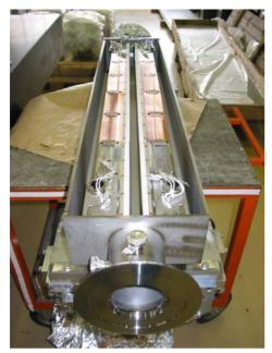
Figure 1: Top view of the open LHC collimator tank with two 1.2 m long CC jaws installed.
