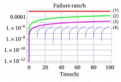
Figure 2: Comparison of designs for safety and consequences on failure rate: one system with constant failure rate (1), two systems in parallel (2) plus surveillance (3) and diagnostics (4).
