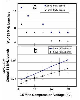
Fig.1. ESME simulations for 8 GeV bunch compression of 2.5 MHz pbar bunches in the MI. a) Number of 53 MHz bunches vs compression voltage and b) 53 MHz LE vs compression voltage.
