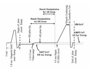
Figure 3: A schematic view of the MI pbar acceleration ramp presently in use. The regions of bunch manipulation at 8 GeV for Recycler and Accumulator pbar injection are also shown. The horizontal dashed indicates the two 8 GeV energies in the MI, one for Recycler and another for Accumulator pbar injection.
