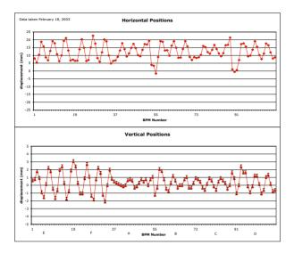
Figure 3: Beam position data from the Tevatron showing difference between two orbits with different average momenta. Horizontal positions above, vertical below.
