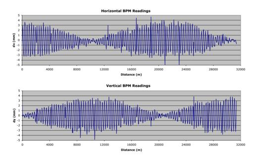
Figure 2: Orbit difference data, taken on February 22, 2003, for 5 consecutive turns. The circumference of the Tevatron is 6283 m. The incoming horizontal oscillation (top) completely couples to the vertical plane (bottom) in  $\sim$ 1.5 revolutions.
