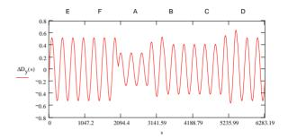
Figure 4: Estimated dispersion pattern generated by skew quad corrector settings and "missing" SQ components.
