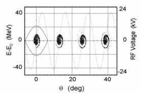
Figure 2: Phase space ( $\Delta E$ ,  $\theta$ ) distribution showing the effect of 2.5 MHz beam loading at injection.
