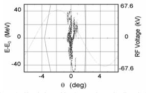
Figure 3: Simulation with 53 MHz beam loading during 2.5 MHz acceleration. Phase space ( $\Delta E$ ,  $\theta$ ) plot shows the first bunch after transition.
