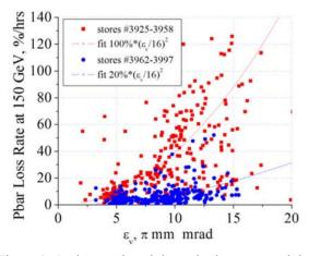
Figure 1: Antiproton bunch intensity loss rates at injection in units % per hour vs 95% vertical emittance  $\varepsilon_V$ .
