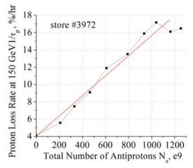
Figure 2: Proton intensity loss rate at 150 GeV helix in units of %/hr vs total number of antiprotons injected into the Tevatron  $N_a$  during shot setup #3972 (February 8, 2005). Points are results of ordinary exponential decay fits over 2 minutes after each antiproton injection. Solid red line is for linear fit  $1/\tau_p[\%/hr]=4+11.6(N_a/1000)$ .
