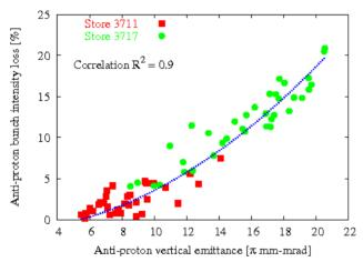
Figure 3: Antiproton bunch intensity loss on the ramp vs antiproton vertical emittance for all bunches in stores #3711(August 5, 2004) and #3717(August 8, 2004). Dotted line represents fit  $dN_a[\%] \approx 20(\varepsilon_a/20)^2$ .
