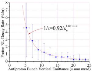
Figure 7: Non-luminous loss rate of proton bunch intensity at the start of stores vs vertical emittance of the correspondingly colliding antiproton bunches.
