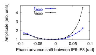
Figure 7: Strengths of two lattice resonances as a function of the horizontal phase advance shift between the two IPs.
