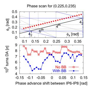
Figure 4: DA for RHIC tunes  $(Q_x,Q_y)=(0.225,0.235)$ , using all arc quadrupoles to vary the horizontal phase advance between the two IPs (bottom). The top plot shows the working point in the phase advance diagram.
