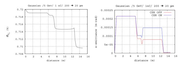
Figure 3: Left: Standard deviation of the relative energy deviation. Right: Normalized transverse emittance (x-emittance).
