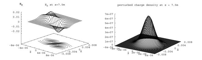
Figure 1: Left:  $E_Z$  at s = 7.5m (end of  $3^{rd}$  magnet of the chicane). Right: Perturbed charge density at s = 7.5m.
