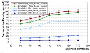
Figure 5: The beam transmission vs. the solenoid current.
