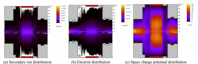
a) Secondary ion distribution (b) Electron distribution (c) Space charge potential distribution Figure 4: The (r,z) distributions of the secondary particles and the space charge potential at the steady regime.
