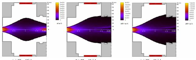
(a) The  $H^+$  beam (b) The  $H_2^+$  beam (c) The  $H_3^+$  beam Figure 3: The (r,z)  $H^+$ ,  $H_2^+$  and  $H_3^+$  beam dynamics at the steady regime of the SCC (after 6  $\mu$ s of computation).
