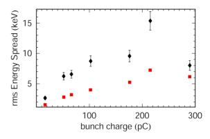
Figure 5: Effective uncorrelated energy spread measured in the GTF (black diamond) and the corresponding theoretical value (red square).
