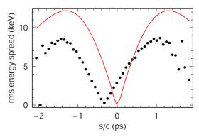
Figure 3: Uncorrelated rms energy spread as a function of bunch position s/c (head at s < 0) from *Parmela* (black symbol) and from Eq. (8) (red curve).
