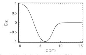
Figure 1: Dimensionless longitudinal field  $\overline{E}(z)$  as a function of distance z from the cathode in the LCLS gun.
