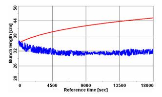
Figure 2: Bunch length with (blue) and without (red top curve) cooling for Cu-Cu collisions of Fig.1.
