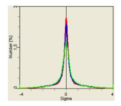
Figure 4: X, Y, and longitudinal profiles after 4 hours of magnetized cooling for Au-Au collisions at 100 GeV/u cooling with number of electrons per bunch  $N_e=3*10^{11}$ .
