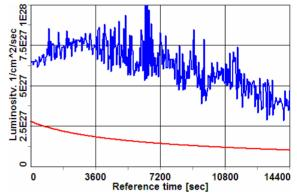
Figure 5: Luminosity with (blue) and without (red) nonmagnetized cooling for Au at 100 GeV/u (112 bunches, 1e9 ions per bunch, normalized 95% emittance 15  $\pi$  um).
