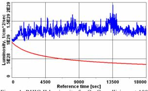
Figure 1: RHIC-II luminosity for Cu-Cu collisions at 100 GeV/u with (blue top curve) and without (red) cooling.
