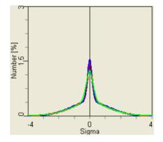
Figure 3: X, Y, and longitudinal beam profiles after 4 hours of magnetized cooling for Au-Au collisions at 100 GeV/u with number of electrons per bunch  $N_e=1.2*10^{11}$ .
