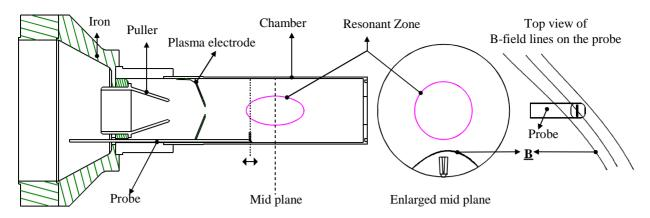
Figure 1: The probe positioning relative to the radial loss cones of the magnetic structure of CAPRICE ECRIS.
