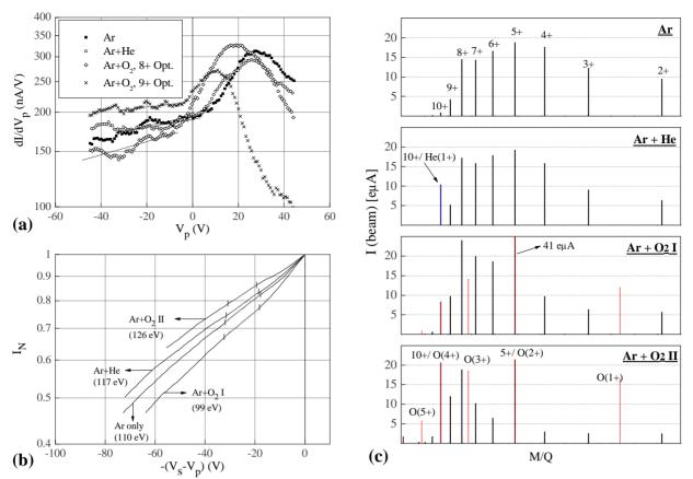
Figure 3: Langmuir probe measurements of (a) plasma potentials, and (b) fast electron temperatures; and (c) corresponding external beam charge distributions (CSD's) for pure Ar, He gas mixed and  $O_2$  gas mixed plasmas.
