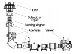
Figure 1: Injection beam line layout. The distance from ECR to analysis magnet is about 2.2 m.
