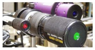
Figure 3: Solid state lasers.
