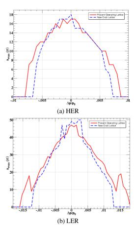
Figure 4: Dynamic aperture of HER and LER with 10% coupling. Solid and dashed lines show the present operating lattice and new crab lattice, respectively.
