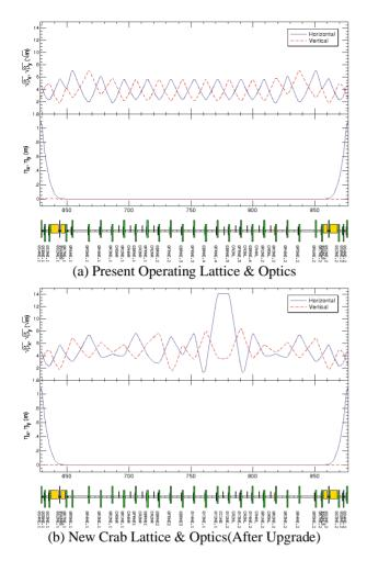
Figure 2: Lattice structure & optics functions of the HER NIKKO section. Electron transits from right side to left side in figure.
