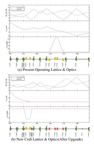
Figure 3: Lattice structure, optics functions and local bump at the upstream of the LER NIKKO section. Positron transits from left side to right side in figure.
