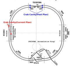
Figure 1: KEKB ring and candidate position for installing crab cavities.
