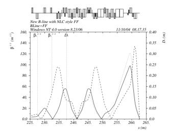
Figure 4: Final focus optics for the new B-Line. (The s-coordinate here is shifted  $\sim 100$  m relative to Fig. 2.)
