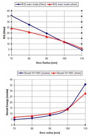
Figure 5: R/Q and stored field energy versus cavity bore.
