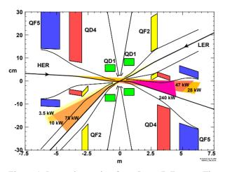
Figure 4: Interaction region for a Super B-Factory. The first quadrupole is at 35 cm from the interaction point.
